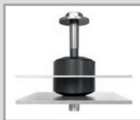
Introduction of the screw through the metal sleeve of the SITEC® Clip and fastening with a weld nut on the rear of the receiving part
