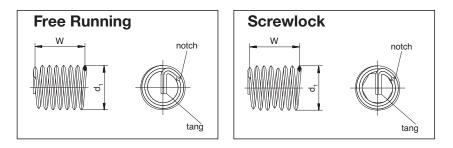
W and  $d_1$  are the control values for thread inserts (Free Running and Screwlock) before they have been installed. The length can only be measured for installed thread inserts.
