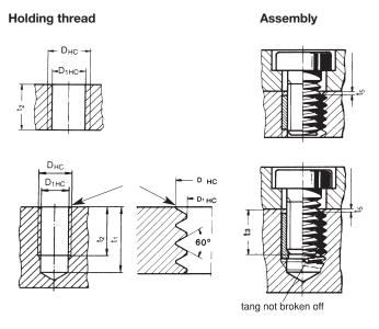
Prior to tapping, counter-bore 90° and deburr. Outside diameter of **countersink** =  $D_{HC}$  + 0.1 mm.
